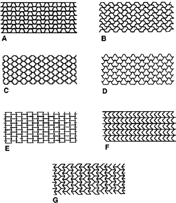
Figure 11-11. Cell configurations for formable paper honeycomb cores.
