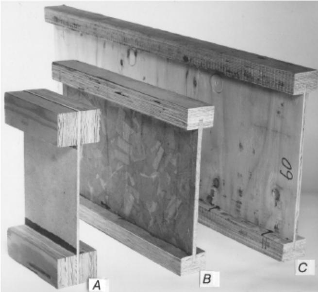
**Figure 11-7. Prefabricated I-joists with laminated veneer lumber flanges and structural panel webs. (A) One experimental product has a hardboard web. The other two commercial products have (B) oriented strandboard and (C) plywood webs.**
